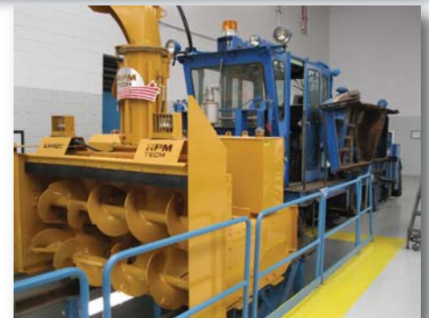
LM220 Detachable Snow Blower Mounted on a Ballast Regulator
