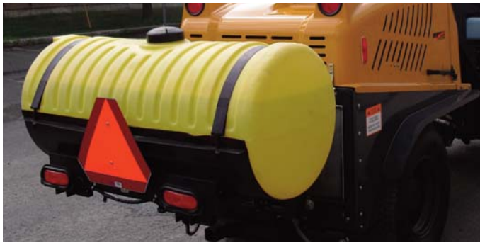
An anti-icing fluid reservoir is available with spraying nozzles located for the customer needs.
