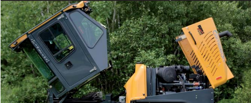
Tilt over cabin and tilt over hood for easy maintenance
